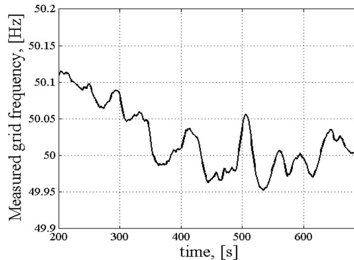
Measurements of the frequency during a day, highlighted the periods where the changes were highest for a 500 second period (for the entire measurement period of close to two months)
