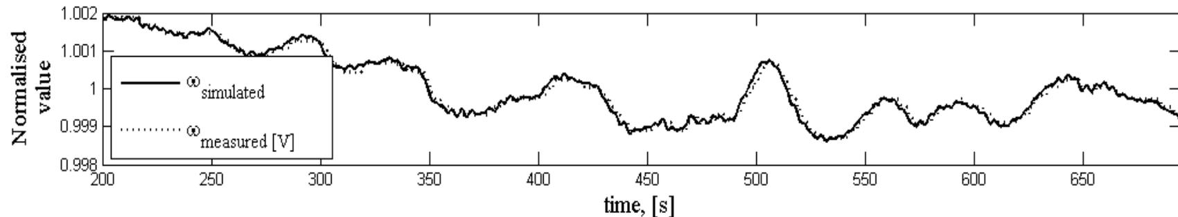
The main conclusion is that the grid frequency volatility should be taken into account when dimensioning the runner
